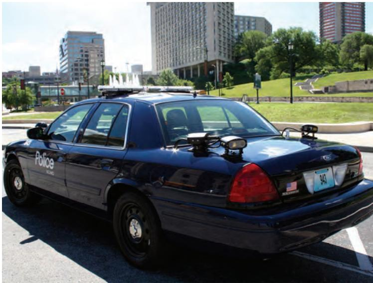
They can take pictures at a distance of about 25 to 30 feet and at highway speeds. One system can run 7,000 license plates a day before the data needs to be moved wirelessly to one of KCPD's servers.
